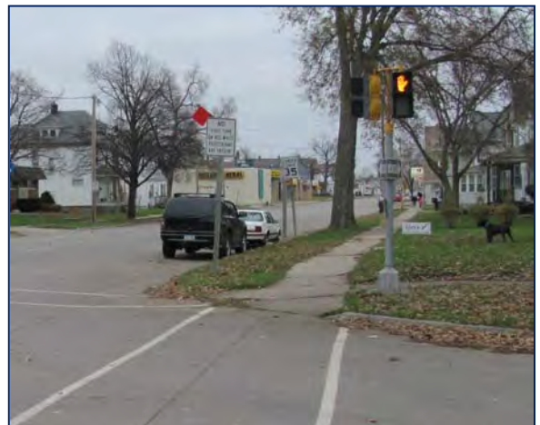
Some signing is in place for "No Right Turn on Red While Pedestrians are Present" at the W. 5th Street and Locust Street intersection.
